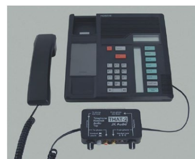
Figure 26: Equipment for testing IVR systems (Barnum, 2011)
